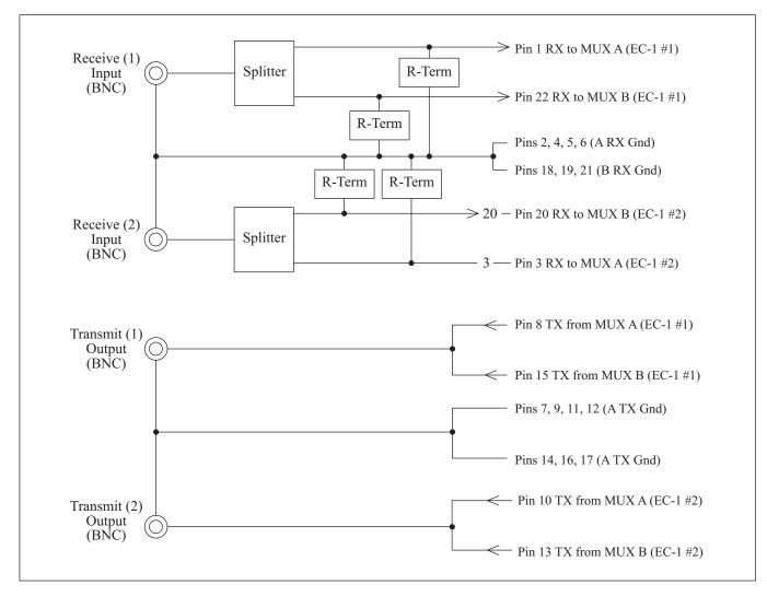
Figure 2. Block Diagram of the Quad BNC Adapter Module
